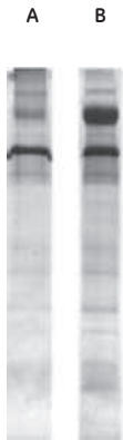
Fig 2.1. Comparison of SDS-PAGE Clean-Up Kit with ethanol precipitation. (A) Urinary protein precipitated with 10 volumes of ethanol. (B) Urinary protein precipitated with SDS-PAGE Clean-Up Kit. Gel: 8 × 9 cm, 12.5% acrylamide, 0.1% SDS, run on SE 260 Mini-Vertical Unit. Stain: Coomassie** Blue R-250.
