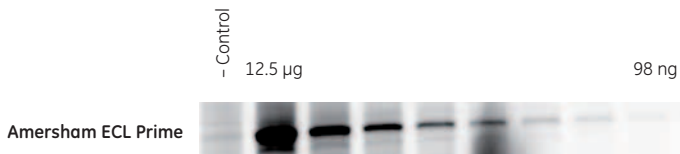
Fig 6.4. Detection of pSTAT3 in IFN \alpha -treated HeLa cells using Amersham ECL Prime. Note that protein quantities refer to the total amount of loaded protein extracted from cell lysate. pSTAT3 comprises only a fraction of that total quantity. The control lane contains 6.25 \mu g of total protein from untreated cells.
